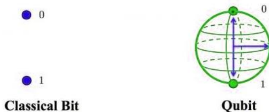
Fig. 3 Basic bit vs. qubit representation
