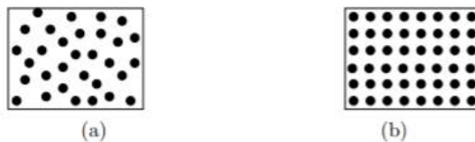
FIG. 15: (a) Particles in liquids do not have fixed relative positions. They fluctuate freely and have a random but uniform distribution. (b) Particles in solids form a fixed regular lattice.
